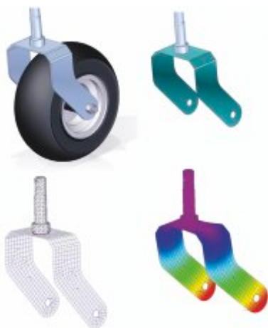
Bridge.asm, Static Study 1 Stress - Elemental Contour: Beam EndA Max Comb Stress Deformation: Total Translation Date: Wednesday, May 19, 2011 10:44 AM
